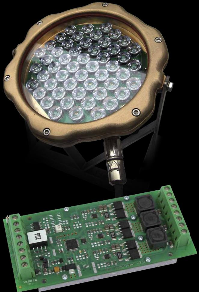
The Aquapaint LED system consists of the following parts: waterproof, high power RGB LED lamp 5300 lumen at 118 watts. waterproof, high power 3 channel LED driver with isolated DMX interface power supply providing a safe system voltage combined cable for both power and DMX
